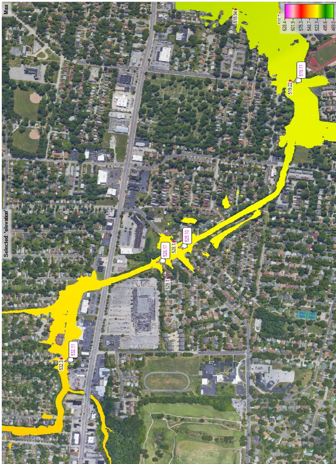
Figure 10. Calibration Results of 2008 High Water Mark Data – West Project Area
